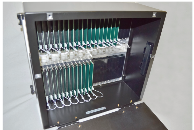
A 50 Module ITA Enclosure Slotted with PCBs
