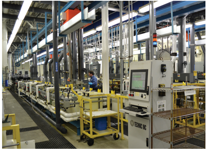
VPC's PLC-Driven Plating and Surface Finishing System.
