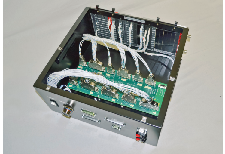
Enclosure with Secondary Connectors and Silkscreen Labels
